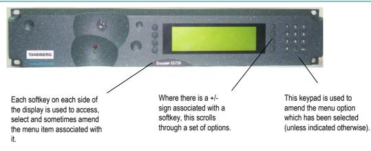
Figure 4.6: 2U Keypad and Display Functions
